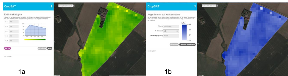
Figure 1 a) Vegetation index is displayed on Google Maps, where the user should enter five levels of N fertilisation compared with the coloured scale. B) VRA file ready to be entered into the fertiliser spreader via a USB memory stick.
